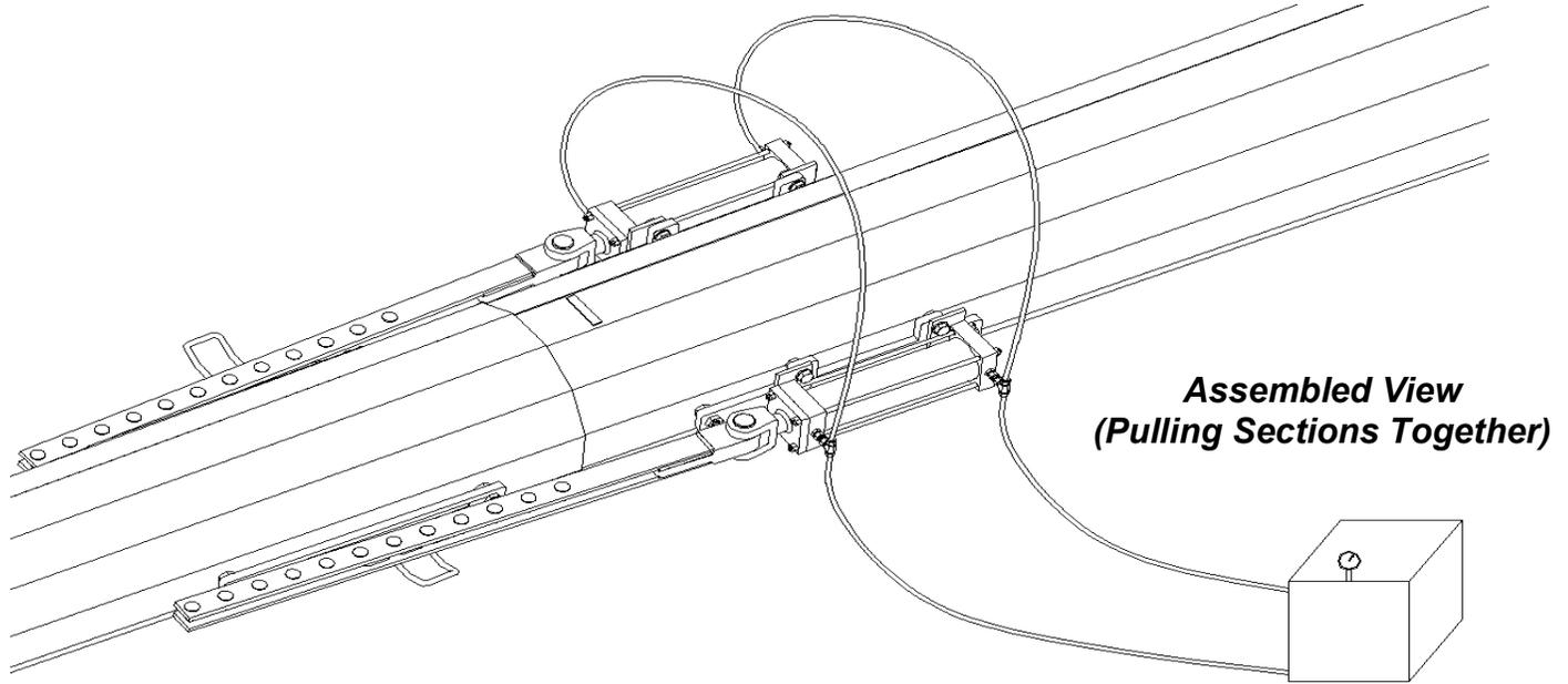
**WARNING:** DO NOT exceed the maximum tandem **pulling** cylinder force (See Valmont drawings). DO NOT exceed maximum operating pressure (3,000 psi). (See Paragraph 3.0 Jacking Device Force Calculation Table)
