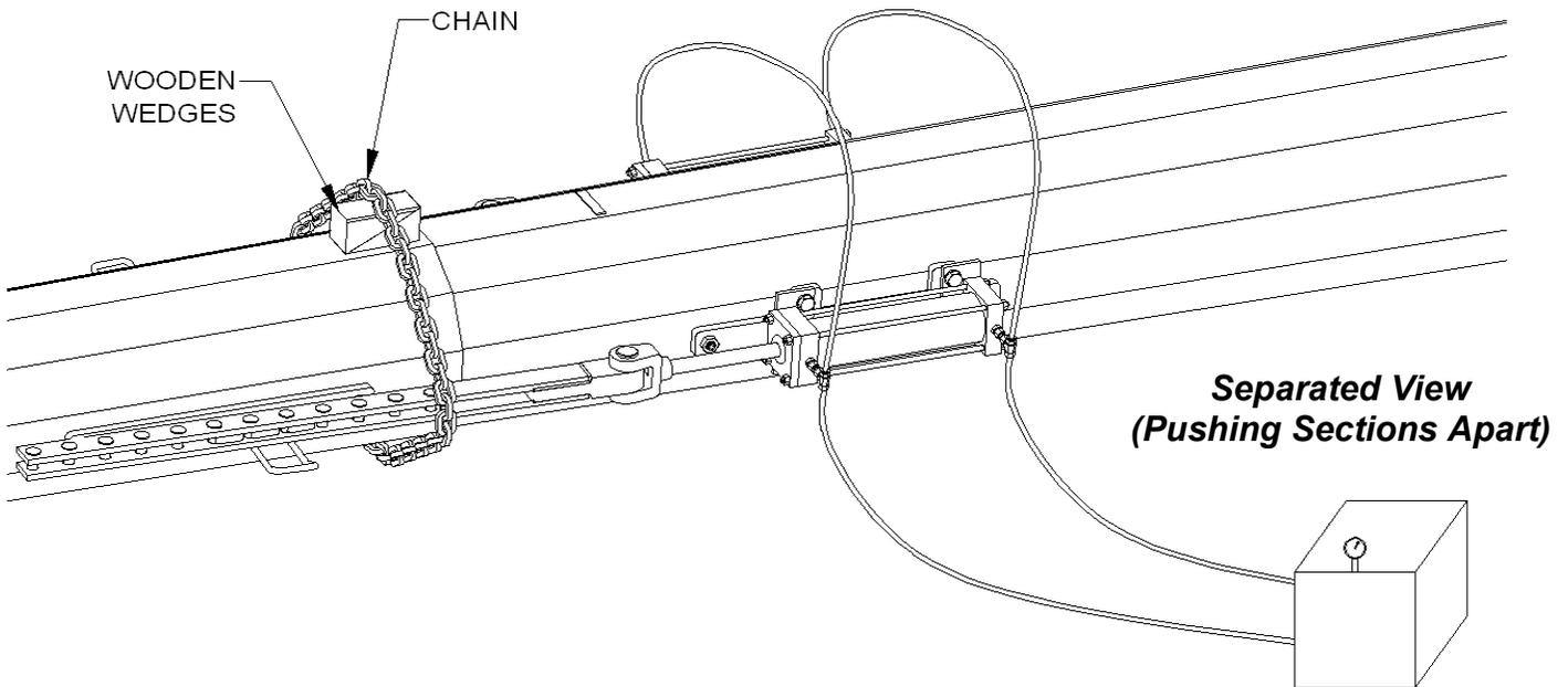
**WARNING:** Chain Push-Pull Bars while separating pole sections to avoid damage to cylinder rod. DO NOT exceed the maximum tandem **pushing** cylinder force (See Valmont drawings). DO NOT exceed maximum operating pressure (3,000 psi). (See Paragraph 3.0 Jacking Device Force Calculation Table)
