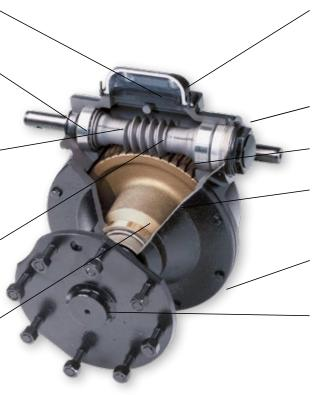
Expansion chamber — Cap made of corrosion resistant cast aluminum; rubber diaphragm allows oil to expand and contract during operation. Vented cap prevents pressure buildup, prevents seal from leaking.
