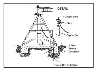
IMPORTANT: All 480 volt AC power supply services MUST be a 4 conductor service. Three 480 Volt AC power lines and one ground conductor which is as large as the power carrying conductors for that service.
