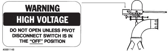
Location: End gun shut off/stop in slot box.
