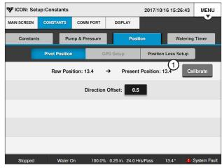
Figure 27-2 Pivot Position Screen 1. Present Position
