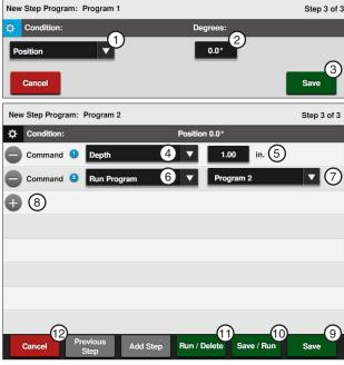
Figure 123-2 1. Position Condition 7. Program 2. Degrees 8. Add Command 3. Save 9. Save 10. Save / Run 4. Depth Command 11. Run / Delete 5. Inches 6. Run Program Command 12. Cancel
