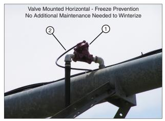
Figure 168-2 1. Aquamatic Valve 2. Plastic Tube
