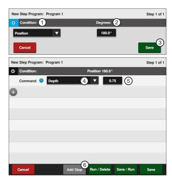
Figure 127-1 1. Position Condition 4. Depth Command 2. Degrees 5. Inches 3. Save 6. Add Step
