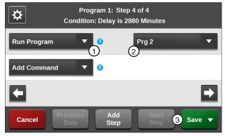
Figure 134-3 1. Run Program Command 2. Choose Command Drop-Down
