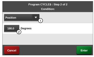
Figure 139-2 1. Position Command 2. Degrees
