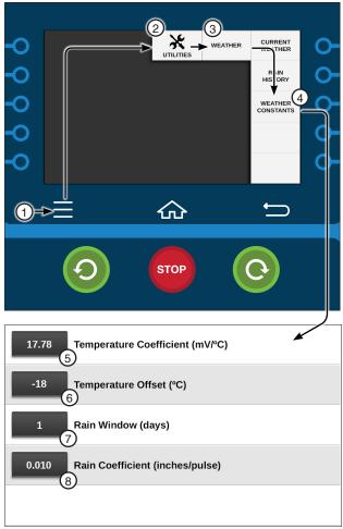
5. Temperature Coefficient Figure 77-1 1. Menu 2. Utilities 6. Temperature Offset 7. Rain Window 3. Weather 4. Weather Constants 8. Rain Coefficient
