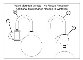
Figure 170-3 1. Aquamatic Valve 2. U-Pipe
