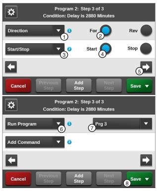
Figure 131-2 1. Direction Command 6. Run Program Command
