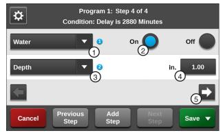
Figure 134-2 1. Water Command 3. Depth Command 5. Next 2. On 4. Inches
