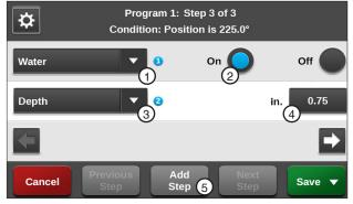
Figure 109-4 1. Water Command 4. Inches 2. On 5. Add Step
