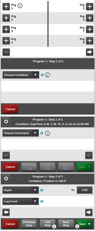
Figure 103-1 1. New Program 4. Add Step 2. Choose Condition Drop-Down 3. Choose Command Drop-Down
