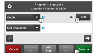
Figure 158-2 1. Depth Command 3. Save 2. Inches Field
