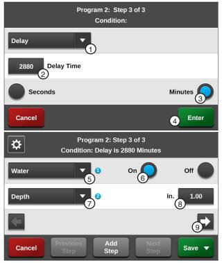
Figure 131-1 1. Delay Condition
