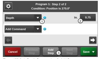
Figure 133-2 1. Depth Command 3. Add Step 2. Inches
