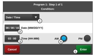
Figure 114-3 1. Date/Time Condition 4. AM 2. Date 5. Fnter 3. Time
