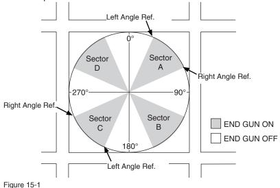
Listed below are typical end gun settings for a pivot, based on the field size and end gun being used. The pivot sectors are based on the location of 0° in relation to the pivot. Refer to Figure 15-1 and the End Gun Settings table below it.
