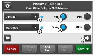
Figure 134-3 1. Direction Command 3. Start/Stop 5. Next 2. Forward 4. Start
