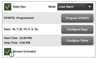
Figure 95-3 Daily Ops Screen 1. Restart Activated Checkbox
