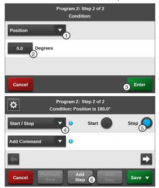
4. Start/Stop Command Figure 130-2 1. Position Condition 5. Stop 2. Degrees
