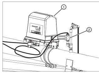
Figure 170-1 1. Aquamatic Valve 2. Plastic Tube
