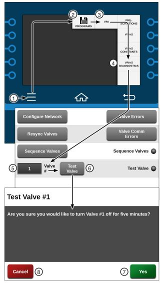
Figure 182-1 1. Menu 5. Valve # 2. Programs 6. Test Valve 3. VRI 7. Yes
