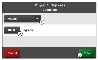
Figure 158-1 1. Position Condition 3. Enter 2. Degrees
