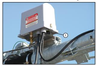
Figure 14-1 1. Disconnect Switch
