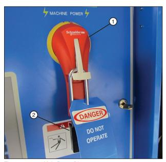
Figure 15-1 1. Main Power Disconnect 2. Lock
