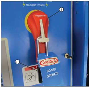
Figure 15-1 1. Main Power Disconnect 2. Lock
