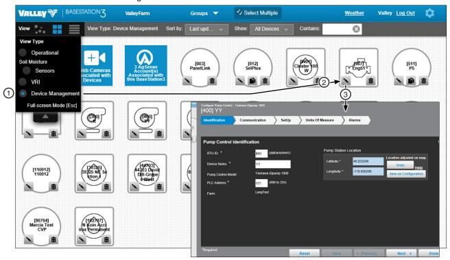
Figure 226-1 1. Device Management View Type 3. Configuration Screen 2. Change Button
