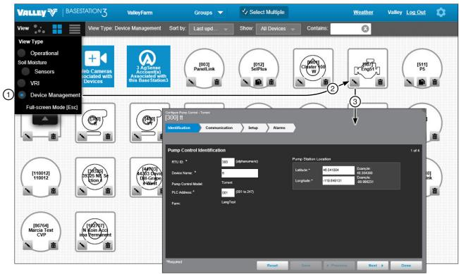
Figure 242-1 1. Device Management View Type 3. Configuration Screen 2. Change Button
