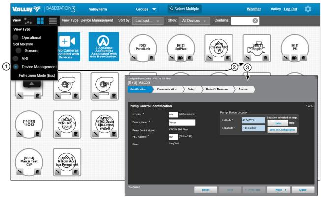
Figure 234-1 1. Device Management View Type 3. Configuration Screen 2. Change
