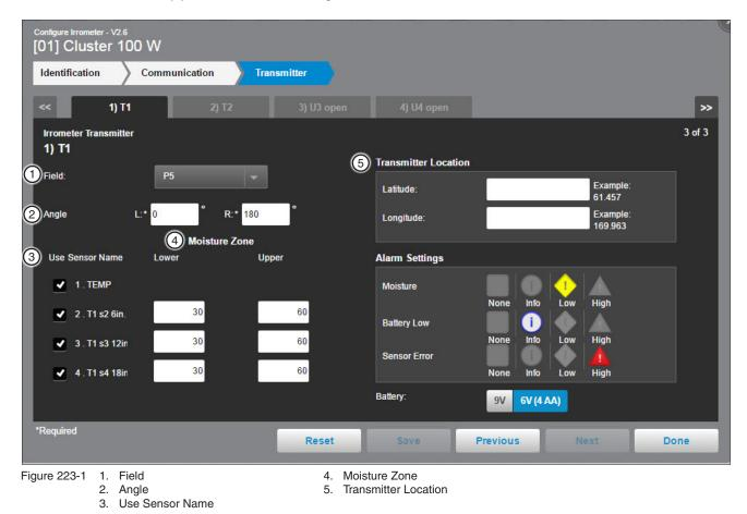
**Transmitter Location (5):** The Latitude and Longitude of the transmitter's location.
