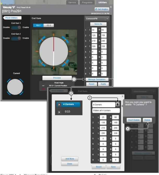
Figure 305-1 1. Manage Templates 2. Select Template Delete
