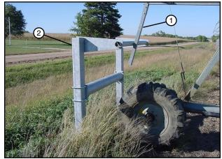
Figure 69-1 1. Actuator Arm 2. Barricade
