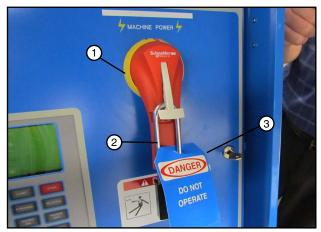
Figure 88-2 1. Main Disconnect 2. Lock 3. Blue OSHA Tag
