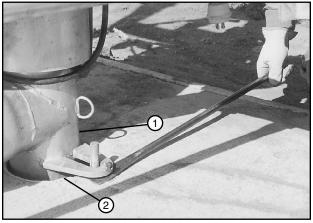
Figure 50-2 1. Riser Pipe 2. Anchor Pipe
