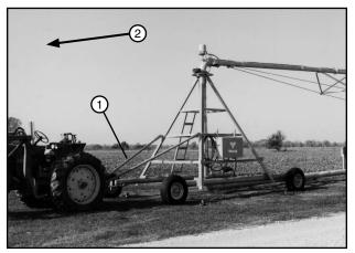
Figure 54-3 1. Tongue 2. Towing Direction
