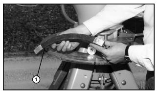
Figure 72-1 1. Rubber Ramp Cut and splice rubber ramps as required.
