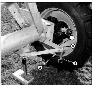
Figure 35-2 1. Steering Arm 3. Torque Pin 2. Tow Link Bar Yoke 4. Lynch Pin
