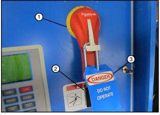
Figure 63-2 1. Main Disconnect 2. Lock
