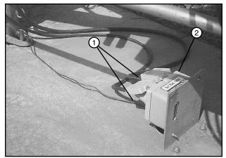
Figure 48-1 1. Power and Pump Control Plugs 2. Receptacles
