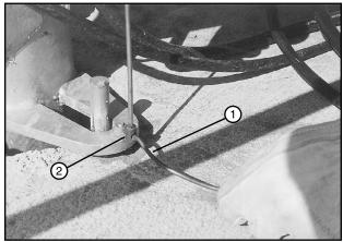
Figure 52-2 1. Ground Wire 2. Ground Lug
