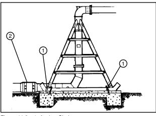
Figure 44-2 1. Anchor Chain 2. Water Supply Line
