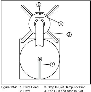
4. End Gun and Stop In Slot Control Box
