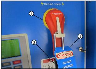
Figure 103-2 1. Main Disconnect 2. Lock 3. Blue Tag
