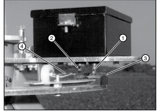
Figure 26-3 1. Stop In Slot Microswitch 2. End Gun Microswitch 3. Stop In Slot Ramp 4. End Gun Ramp
