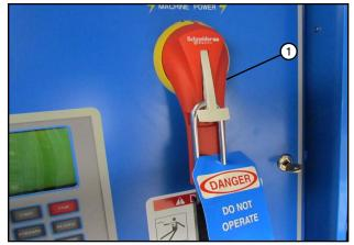
Figure 53-3 1. Main Power Disconnect Series 8000 Control Panel Shown
