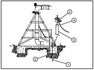
Figure 13-2 1. Ground Rod Installation 4. Copper Ground Wire 2. Service Conductor 5. Clamp 3. Copper Ground Rod
