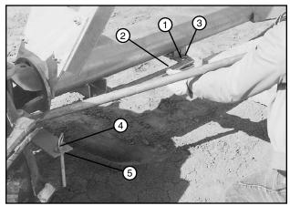
Figure 51-2 1. Carrier Spring 4. Torque Pin 2. Tow Link 5. Steering Arm 3. Tow Link Carrier
