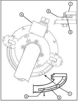
Figure 76-1 1. Stop In Slot Ramp (placed on outside of ring) 2. Mounting Ring
