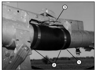
Figure 70-1 1. Flex Hose 2. Hose Clamp 3. Bonding Ground Wire
