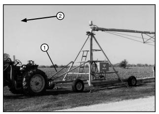
Figure 58-3 1. Tongue 2. Towing Direction
