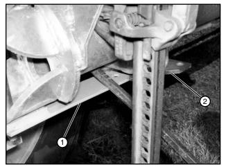
Figure 38-3 1. Steering Arm 2. Latch Plate
