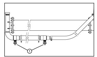
Figure 90-1 1. Booster Pump Hose Drain
