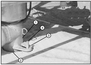
Figure 51-1 1. Riser Pipe 3. Slotted Ear 2. Anchor Pipe 4. Stud
