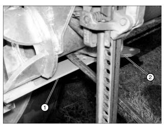
Figure 34-2 1. Steering Arm 2. Latch Plate
