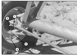
Figure 51-3 1. Steering Arm 3. Torque Pin 2. Tow Link Bar Yoke 4. Lynch Pin
