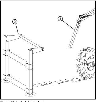
Figure 28-1 1. Actuator Arm 2. Barricade
