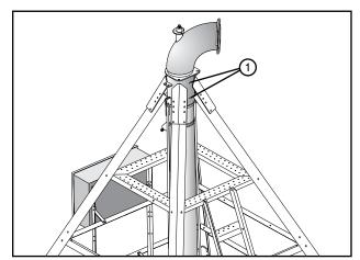
Figure 70-3 1. Grease Fitting
