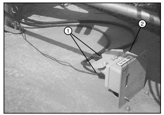
Figure 52-3 1. Power and Pump Control Plugs 2. Receptacles
