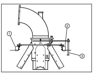
Figure 29-1 Standard Center Pivot Mounted Auto Reverse 1. Reversing Switch
