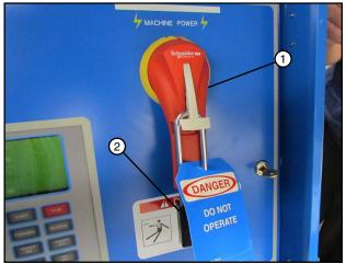
Figure 14-1 1. Main Power Disconnect 2. Lock
