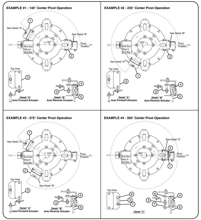
Figure 78-1 1. Auto Forward (Reverse to Forward Actuator- Bolt Down) 2. Auto Reverse (Forward to Reverse Actuator- Bolt Up) 3. Actuator Plate
