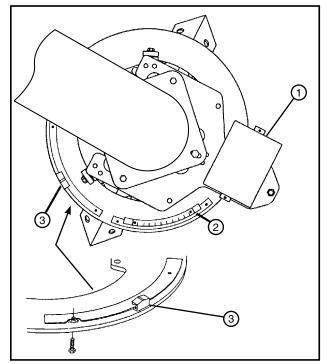
Figure 73-1 1. End Gun and Stop In Slot Control Box 2. End Gun Shut Off Ramp (on inside of ring) 3. Stop In Slot Ramp (on outside of ring)
