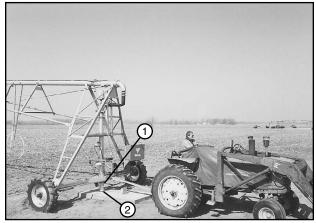
Figure 50-3 1. Riser Pipe 2. Anchor Pipe
