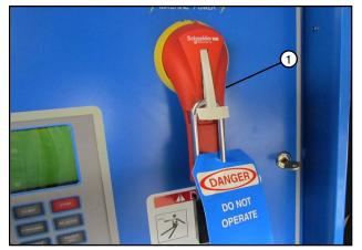
Figure 41-3 1. Main Power Disconnect Series 8000 Control Panel Shown
