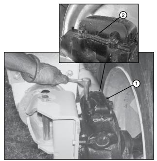
Figure 66-2 1. Expansion Chamber Cap 2. Vent Hole
