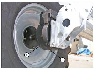
Figure 64-1 1. Wheel Gearbox 2. Drain Plug
