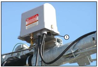
Figure 13-1 1. Disconnect Switch
