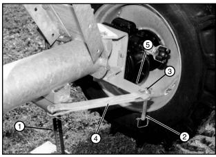
Figure 37-3 1. Jack 2. Lynch Pin 3. Torque Pin
