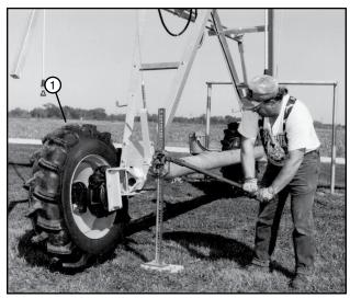
Figure 39-3 1. Tire Shown In Operating Position
