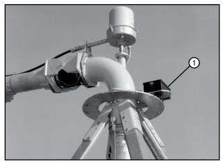
Figure 26-2 1. Stop In Slot / End Gun Control Box
