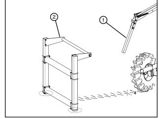
Figure 31-2 1. Actuator Arm 2. Barricade
