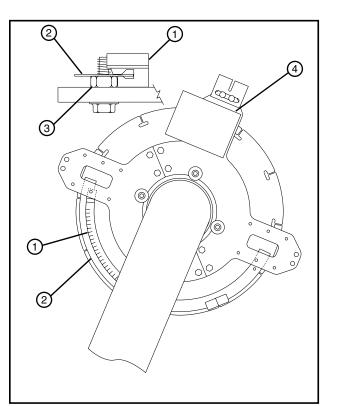
Figure 75-1 1. End Gun Ramp (placed on inside of ring) 2. Mounting Ring
