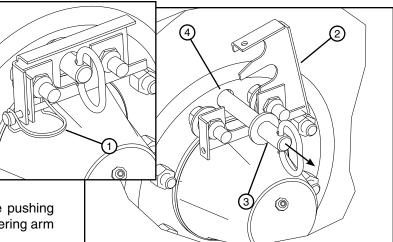
Figure 34-1 1. Lynch Pin 3. Torque Pin 2. Retainer Clip 4. Hub Torque Pin Receiver
