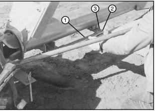
Figure 49-3 1. Tow Link Bar 2. Tow Link Carrier 3. Carrier Spring
