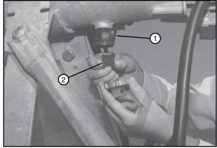
Figure 89-1 1. Pipe Drain 2. Rubber Seal
