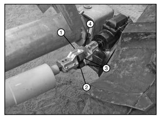
Figure 38-2 1. Drive Shaft U-Joint Half
