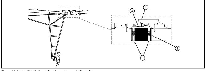
Figure 22-2 1. Hitch Ball and Cup Assembly 3. Band Clamp 2. Flexible Hose 4. Bonding Ground Wire
