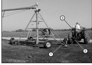
Figure 59-3 1. Tongue 2. Chain 3. Towing Unit
