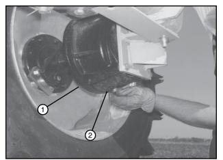
Figure 66-1 1. Wheel Gearbox 2. Drain Plug
