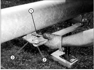
Figure 35-1 1. Carrier Spring 3. Tow Link Carrier 2. Tow Link Bar
