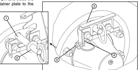
Figure 39-2 1. Hub Torque Pin Receiver 4. Retainer Clip 2. Torque Pin 5. Lynch Pin 3. Retainer Plate
