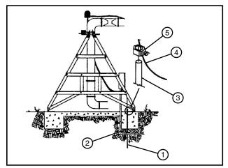
Figure 70-2 1. Ground Rod Installation 4. Copper Ground Wire 2. Service Conductor 5. Clamp 3. Copper Ground Rod
