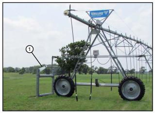
Figure 29-3 1. End of Field Stop Barricade
