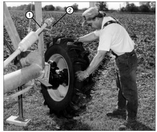
Figure 34-3 1. Drive Shaft 2. Drive Shaft Keeper
