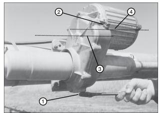
Figure 67-1 1. Drain Plug 3. Oil Level 2. Fill Plug 4. Bottom of Fill Plug Hole
