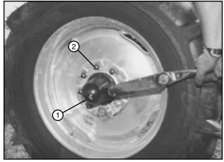
Figure 68-1 1. Grease Fitting 2. Wheel Lug Nut
