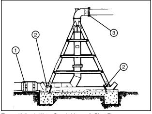
Figure 42-2 1. Water Supply Line 3. Pivot Flex 2. Anchor Chain
