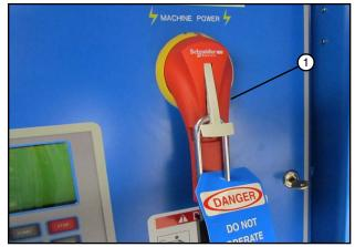
Figure 57-3 1. Main Power Disconnect
