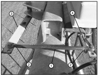
Figure 83-2 1. Connection Rod 3. Control Bar 2. Jam Nut 4. Switch Pivot Arm
