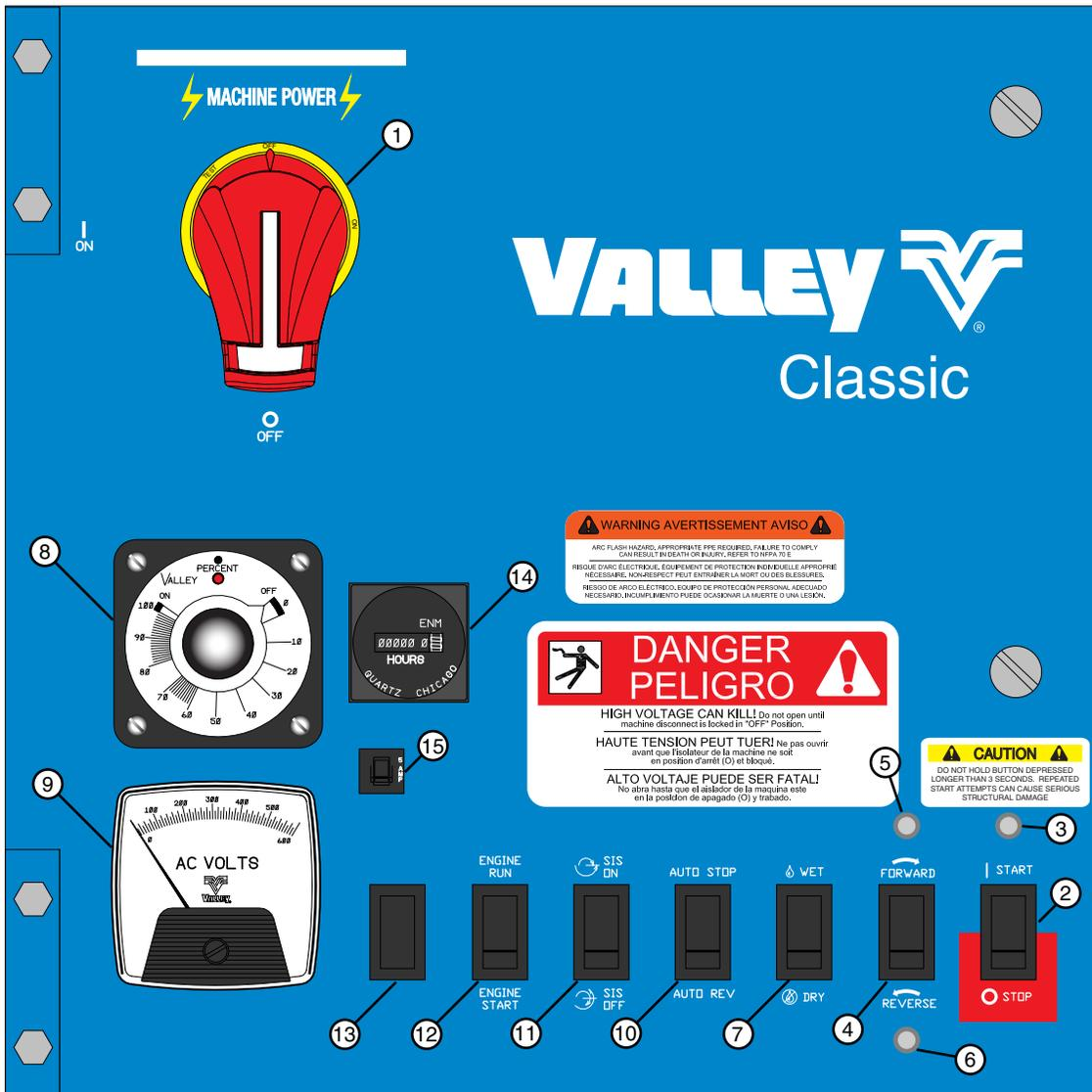
Figure 19-11. Main Disconnect Switch
