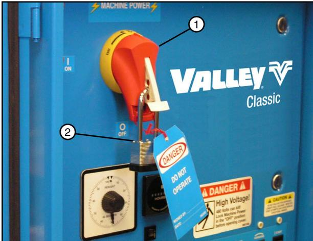
Figure 13-1 1. Main Power Disconnect
