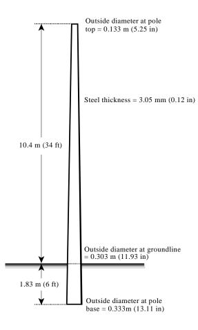
Figure 1. 40 ft class 3 steel pole.
