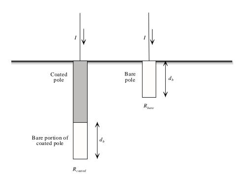
Figure 4. Illustration of *R*<sub>bare</sub> as the upper limit on *R*<sub>coated</sub>.
