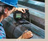
Full penetration welds are always inspected and verified ultrasonically. The component does not progress to the next phase of fabrication until it passes competely.
