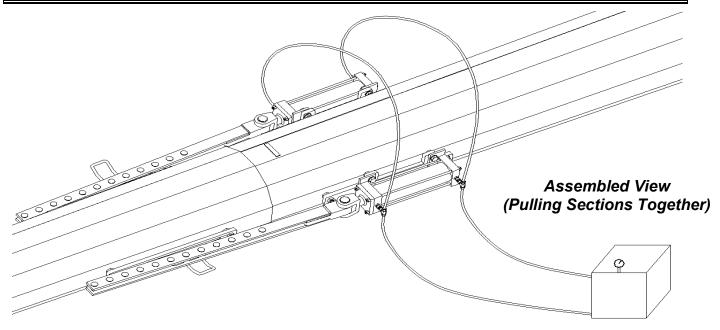
**WARNING:** DO NOT exceed the maximum tandem **pulling** cylinder force **(See Valmont drawings)**. DO NOT exceed maximum operating pressure (3,000 psi). **(See Paragraph 3.0 Jacking Device Force Calculation Table)**
