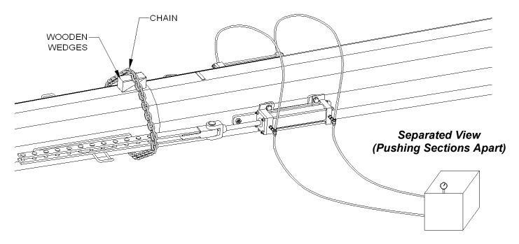
**WARNING:** Chain Push-Pull Bars while separating pole sections to avoid damage to cylinder rod. DO NOT exceed the maximum tandem pushing cylinder force (See Valmont drawings). DO NOT exceed maximum operating pressure (3,000 psi). (See Paragraph 3.0 Jacking Device Force Calculation Table)
