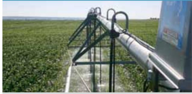
**Details:** The new longer span options help reduce the overall per acre installed cost by reducing the number of drive units needed. These 8000 series, 225-foot spans can also help to reduce the number of wheel tracks in the field for growers with track-prone land conditions. To learn more, talk with your local Valley dealer to find the best combination for your operation.
