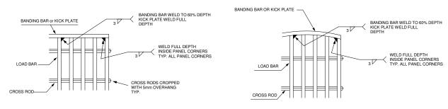
WELD ONE SIDE OF EVERY 5th LOAD BAR FOR A & B PATTERN
