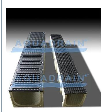
Aquadrain® polymer concrete drainage channels are manufactured from a blend of fine aggregates and a high quality formulated resin used as a binder. By batching these products together under the correct conditions such as temperature and moisture controls, as well as a clean environment, the polymer concrete product is produced. The resin binder used in our polymer concrete channels takes the place of what cement does in a traditional concrete mixture.
