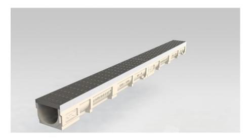
Aquadrain<sub>®</sub> galvanised series polymer concrete channels come complete with galvanised edge rails and a great range of galvanised grates to choose from. After concrete encasement this channel and its associated grates have been tested to a class D loading (210Kn).
